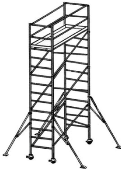
Rolling scaffold with outrigger stabilizers
